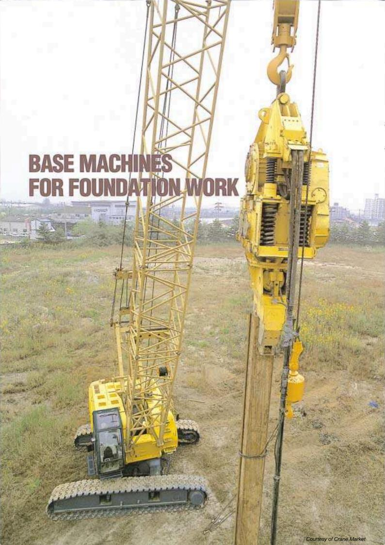
Crawler cranes are being used more and more as base machines for foundation work in urban redevelopment and other large scale projects. Foundation work requires good winch capability, rather than the lifting capability important in crawler cranes used for building construction. These base machines must also exhibit a performance that matches the special characteristics of foundation work processes, such as diaphragm wall digging or cast-in-place pile insertion.
